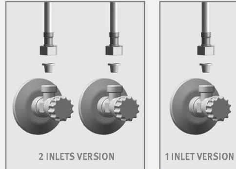
**MAKE SURE THAT THE FILTER(S) IS/ARE INSTALLED BETWEEN THE FLEXIBLE PIPE AND THE SHUT OFF VALVE (ANGLE VALVE) (NOT SUPPLIED).**
